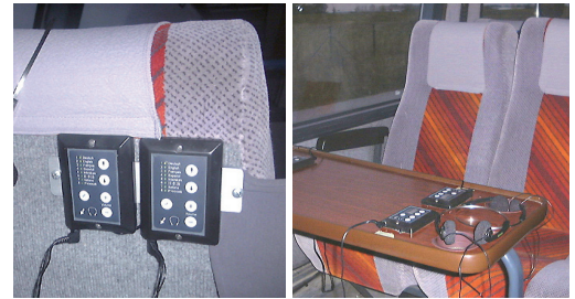
Samples of the seat modules in the field: either on the back side of the seats, or he busses side wall, or on the tables.
